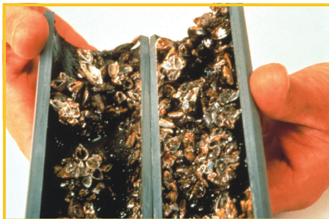
Eurasian Mussels can colonize and clog intake pipes up to 24 inches in diameter Photo: Don Schloesser, USGS
