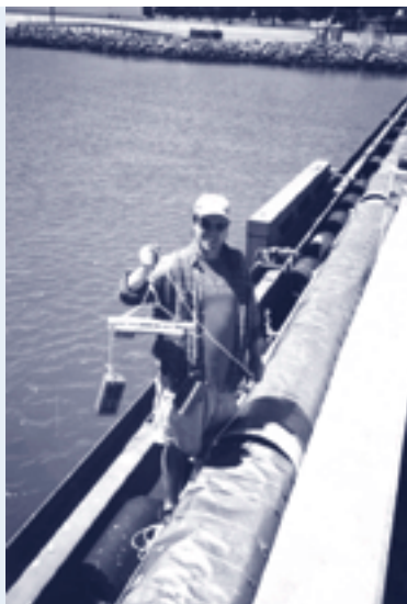
Fouling panels being deployed at Treasure Island in San Francisco Bay. Photo courtesy of SERC.
